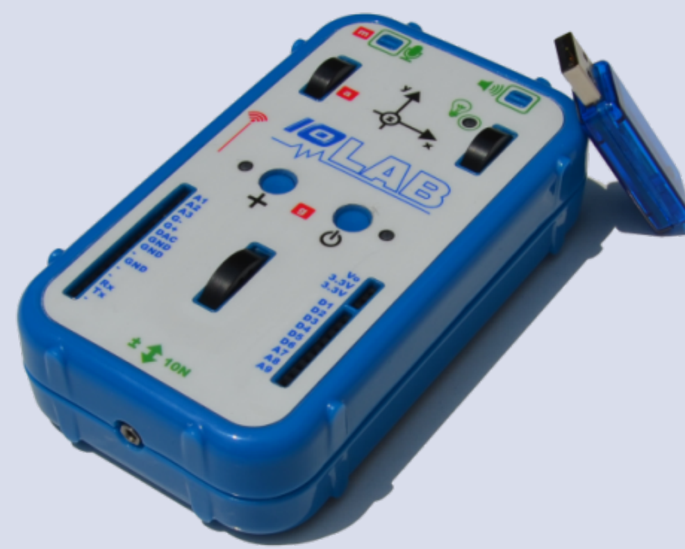
FIGURE 1. The IOLab, version 2, shown with USB dongle. Near the top of the unit are the microphone and speaker, as well as axes for alignment. The three wheels are connected to an encoder. Near the bottom of the unit are the analog and digital inputs and outputs (similar to an Arduino Uno).
